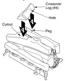
Figure 24 - Installing Crossover Log (#4) [18" Variable Manually-Controlled Set Shown]
